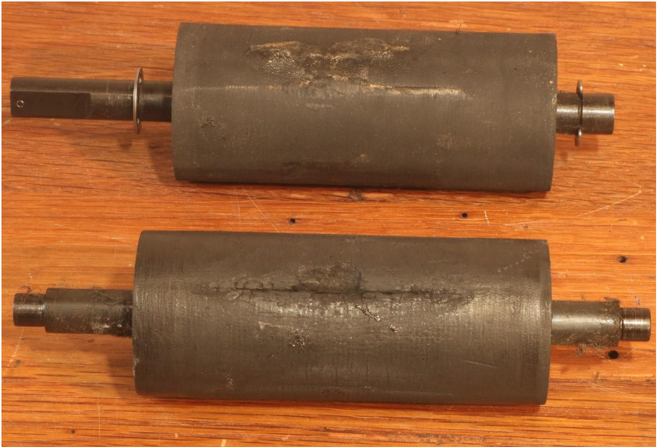
Figure 12: Rollers in poor condition. Top: melted plastic stuck onto bottom roller (part AM4-7a). Bottom: Top Roller (AM4-6a) split from heat. The heat guards on this machine were removed, and heat was left on without machine running, leaving the roller to face the heater block on this side until the rubber degraded. The top roller can be repaired; the bottom one cannot.
