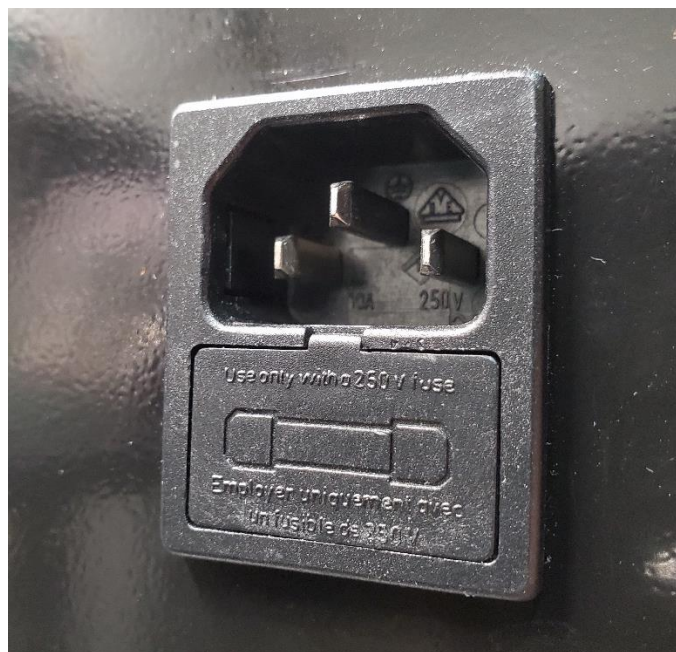
Figure 24: Location of fuse tray under power receptacle.
