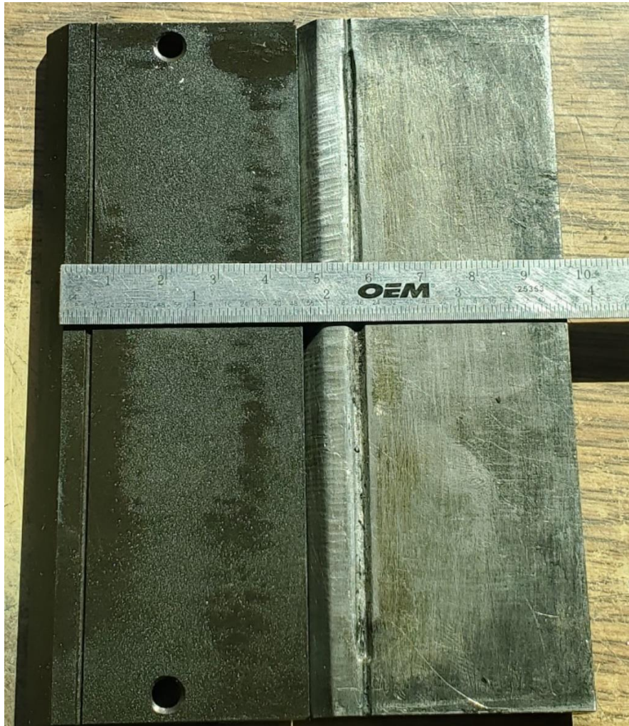
Figure 15: top view of two cutting plates, a new one on the left, and a used one with a badly worn groove on the right.
